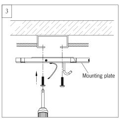
Use metal outlet box suitable for fan support and use only the screws provided with the outlet box (must support 35 lbs). Before attaching fan to outlet box, ensure the outlet box is securely fastened by at least two points to a structural ceiling member (a loose box will cause the fan to wobble). Remove the two outlet box screws provided with the box, aligning the holes of the mounting plate with the holes of the outlet box. Reinstall the 2 outlet box screws securely.
