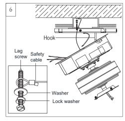
Hang motor assembly onto the hook on mounting plate for hands-free wiring and safety cable installation.
