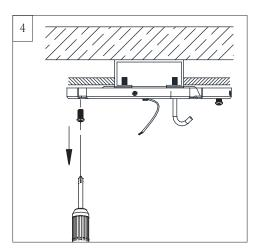
Loosen 2 screws across from each other and remove the other 2 preassembled screws from mounting plate (Corresponding to installation step 8). Save screws for later use.
