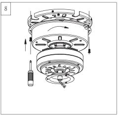
Lift motor assembly, aligning the keyhole slots with the preassembled screws on mounting plate, and twist clockwise till lock. Reinstall the screws removed in step 4. Tighten all screws securely.
