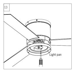
Attach light pan onto the plate on motor, aligning the keyhole slots on the light plate with the preassembled screws on the plate. Twist clockwise till lock. Reinstall the screw removed in step 12. Tighten all screws securely.
