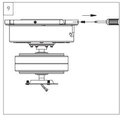
Loosen 2 screws across from each other and remove the other 2 preassembled screws from side of mounting plate (corresponding to installation step 10). Save screws for later use.
