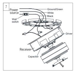
Make wiring connections using wire connectors provided as indicated above. White from house to White from remote receiver marked AC N. Black from house to Black from remote marked AC L. Connect all green grounded wires to Grounded wire from House. Make sure that no filaments are outside of the wire connector.
