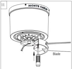
Install blade with screws provided, aligning each of the holes as shown and tighten all screws securely. Repeat this process for remaining blades.
