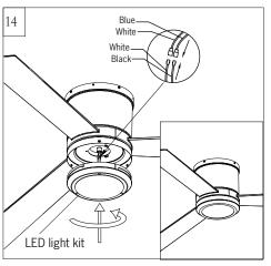
Connect white wire from fan to white wire from LED light kit and then connect blue wire from fan to black wire from LED light kit.
